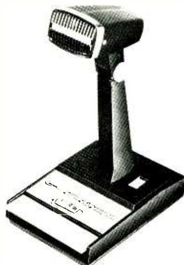
selection of relay or electronic switching. Press-to-talk bar may be locked in talk position. Frequency response is 100-8000 Hz; impedance is 1000 ohms; cable is six-foot; three-conductor coiled cord with plug.—**Fanon/Courier Corp.**, 990 South Fair Oaks Avenue, Pasadena, Calif. 91105.
