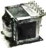
G.E. 9T56Y8831, rated at 2.09 K.V.A. 7 taps, 14, 23.5, 105, 110, 115, 120, and 125 volts. Input voltage any voltage from 105 to 125 volts. Output voltage any of the tap voltages above. Currents in excess of 15 amperes per tap. Ideal for raising or lowering line voltages, and getting 14 or 23.5 volts at high current as well. Many other voltage combinations possible. We supply data sheet showing many voltages possible with this transformer. In original factory cartons. Weight 12 lbs. ea.
