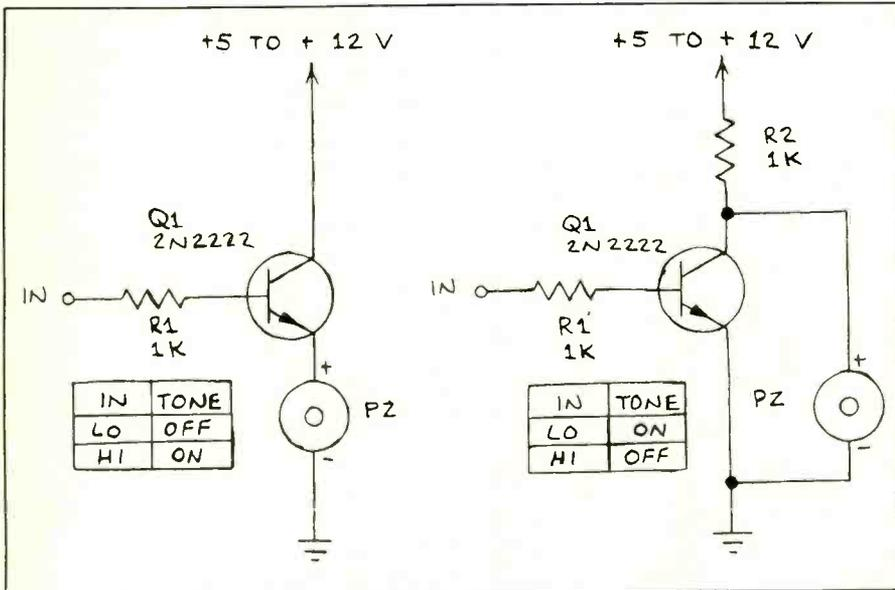
Fig. 6. Piezoelectric buzzer logic interfaces.
