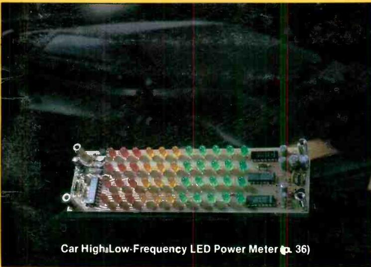
Car High/Low-Frequency LED Power Meter (p. 36)
