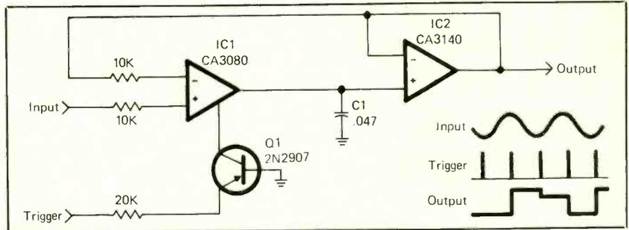
Fig. 5. A typical OTA sample/hold circuit.
