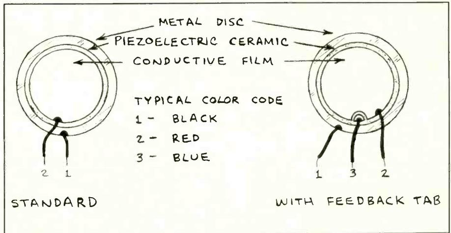
Fig. 1. Details of typical piezoelectric buzzer elements.
