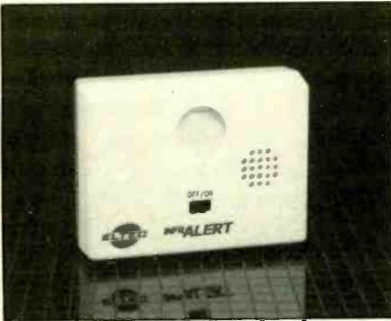
The device is powered for up to a year by a single 9-volt battery. It uses fixed-focus optics that give it a narrow field of view that is less likely to interfere with normal room activities than is possible with wide-field-of-view systems. Its built-in delay circuit gives you time to arm the system and leave the protected area without tripping the alarm.
