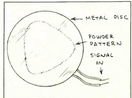
Fig. 2. Nodal pattern of an oscillating piezoelectric buzzer element.
