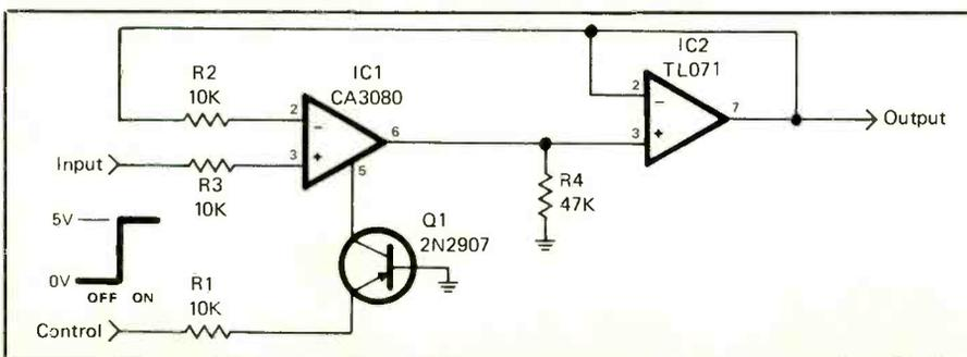
its input when triggered and continues to "hold" that level until another command is issued. When the control line goes high, the *IC1* OTA acts as a closed switch and charges *C1* until the input and output voltages are equal. With the line low, the "switch" opens so that the voltage is stored in *C1*. To prevent leakage currents from introducing errors, use a low input bias operational amplifier like the CA3140 or LM351 for *IC2* and polyester or polystyrene capacitor for *C1*.
