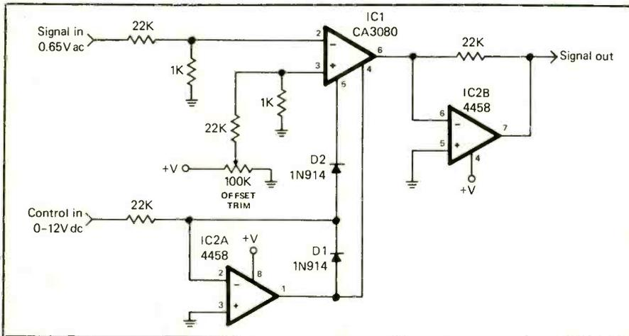
Fig. 3. Improved voltage-controlled amplifier uses ordinary operational amplifiers as a voltage-controlled circuit source and an output buffer.
