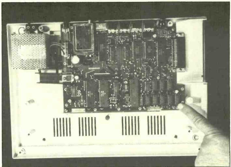
*Eight socketed memory ICs are in the lower-right of the motherboard. Remove the factory-installed 16K chips and replace them with 64K chips.*
