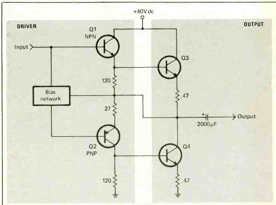
Fig. 11. The "quasicomplementary" circuit uses the same type of npn and pnp transistors in a totem-pole arrangement and a complementary driver stage consisting of  $Q1/Q2$ .
