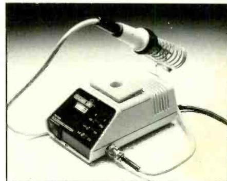
The tri-temperature station uses J-type thermocouple sensing to provide stable and accurate temperature repeatability within ± 5 degrees Fahrenheit. The CMOS-safe plug-in soldering iron features a comfortable, cool grip and a non-burn cord. It includes the soldering station with switches and indicators, soldering iron, long-life tip and tip cleaning sponge. Both 117- and 230-volt ac models are available, each with 24-volt, 48-watt handpieces.
