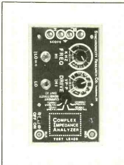
sible for the CIA to perform accurate inductance and capacitance measurements from less than 2 mH to beyond 200 H and from less than 100 pF to beyond 20 μF. The impedance of complex networks and transducers can also be measured. The CIA is battery powered for convenient field-service use, but it can also be used on a testbench.
