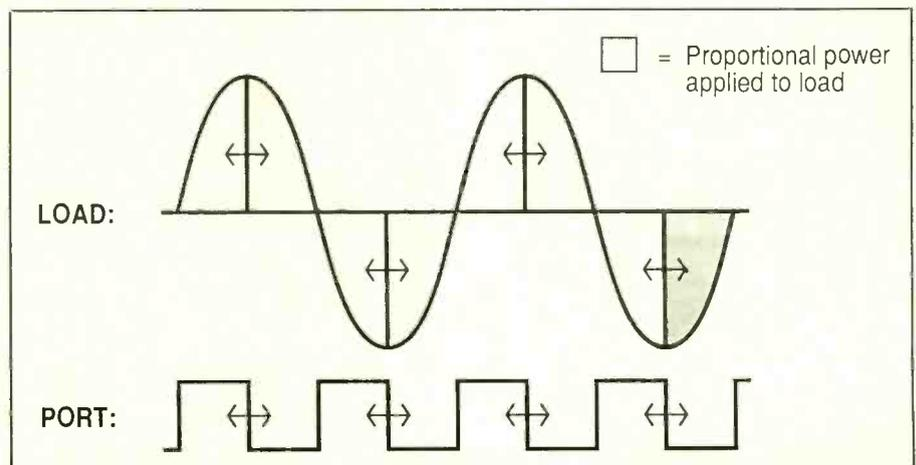
Fig. 4. Proportional power control requires precise timing.
