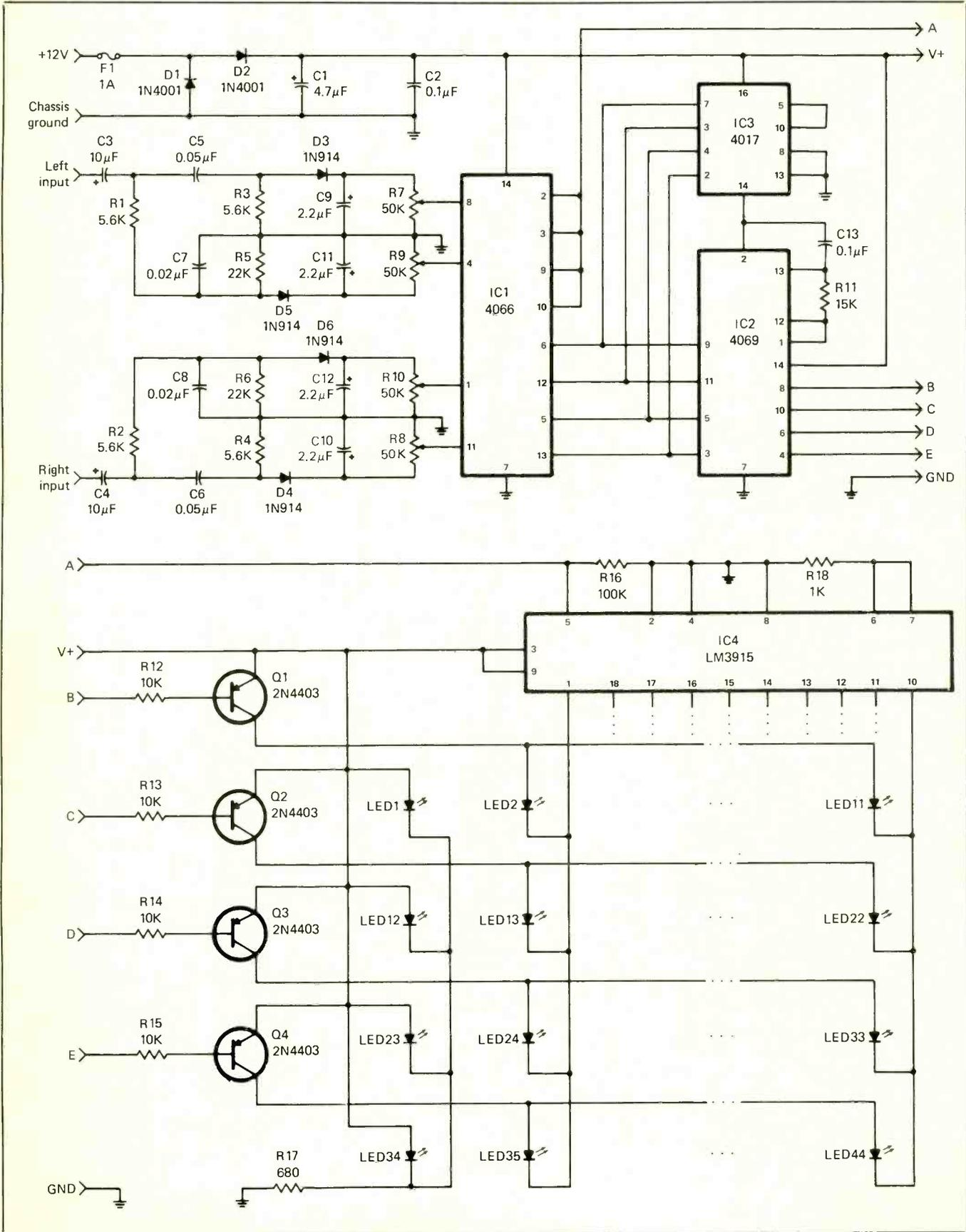
Fig. 2. Separate high- and low-frequency "bar" displays consist of 10 LEDs in each channel bar, plus one LED in each bar that comes on when dc power is applied. Only four LEDs are shown for each channel.
