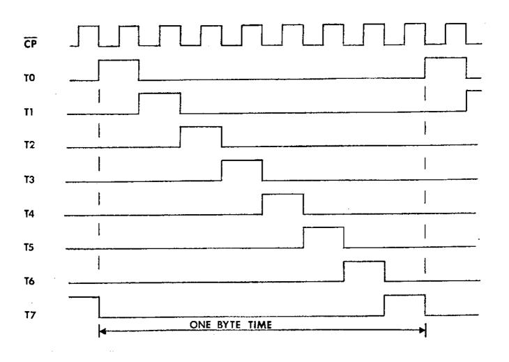
A byte time lasts eight bit times, from the start of TO to the next start of TO.
